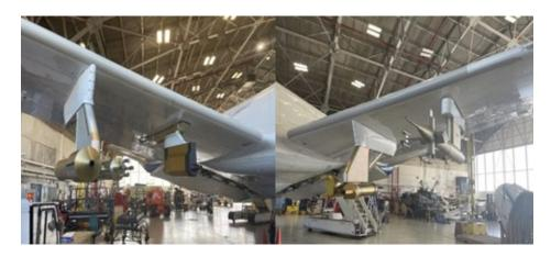
The left and right wings of the P-3 aircraft capture data in different ways, some particles entering directly into their openings, some read by lasers, and more. Photo Credit: Christian Nairy.
